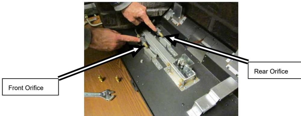
6. Install the LP pilot orifice following the directions below.
