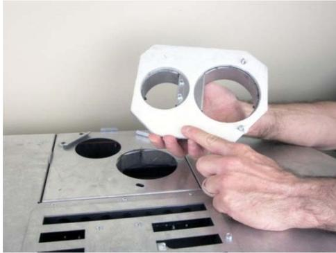
5. Attach the 4" exhaust vent to the connector and secure with at least 3 screws.
