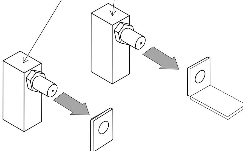
4. Remove and discard the stock seal plates. Install the LP seal plates as shown below.
