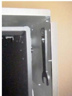
**NOTE:** Replace the tool in this location after removing the glass frame.
