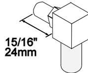
Apply thread sealant to the LP orifices prior to installation. Use the chart below to identify the correct orifices.
