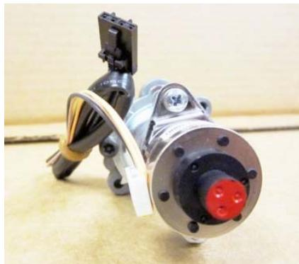
9. Restore the appliance to the correct configuration. Make the gas line connection, bleed the gas line (if applicable), start the heater and thoroughly leak-test all gas connections and the gas control valve.
