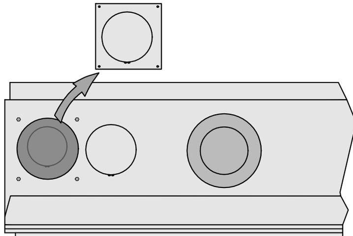
2. Use snips or diagonal cutters to snip the tab on the knockouts. Press on the far side away from the tap to pop the edge of the knockout up. Grab on to the knockout with pliers and bend it back and forth until the remaining tabs break free. Discard the knock out plate. The power heat duct is now ready to install (see kit instructions for details).
