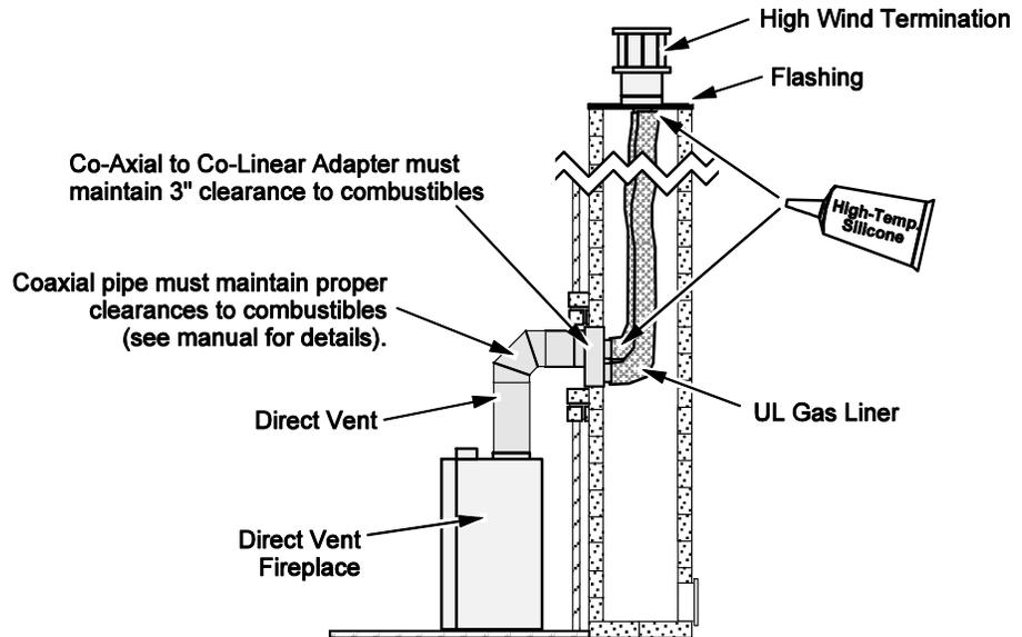
This appliance may utilize 6-5/8" diameter direct vent manufactured by Duravent (reducer may be required). The vent may be adapted to utilize an existing masonry fireplace using the Duravent Masonry Chimney Conversion Kit (part # 46DVA-KMC). The vent must be installed following all directions included with the vent and those listed below:
