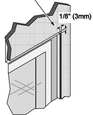
**!** Make sure the seams on the non-combustible board is to the sides or below the glass opening (do not place seams on corners of glass, especially the upper corners).
