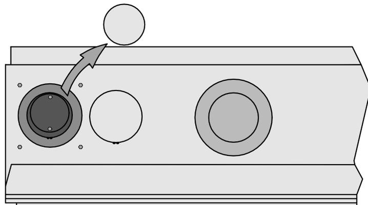
3. Under the second layer of knockout plates, you will find cover plates held in place with (2) 1/4" screws. Use a nut driver or drill with an extension to remove the (2) screws. Reach in and remove the cover plate. You may discard the plates
