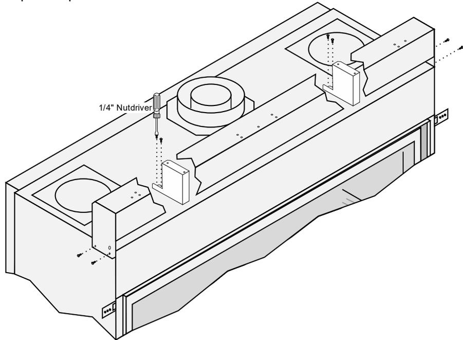
**WARNING:** For flush installations, combustible facing can touch the first  $\frac{1}{2}$ " of the fireplace box. **ONLY NON-COMBUSTIBLE FACING** can cover the front of the appliance.
