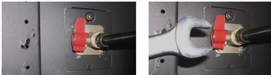
2. Remove the screw that holds the shutoff valve plate in place (1/4" nutdriver). Remove the shutoff valve plate.
