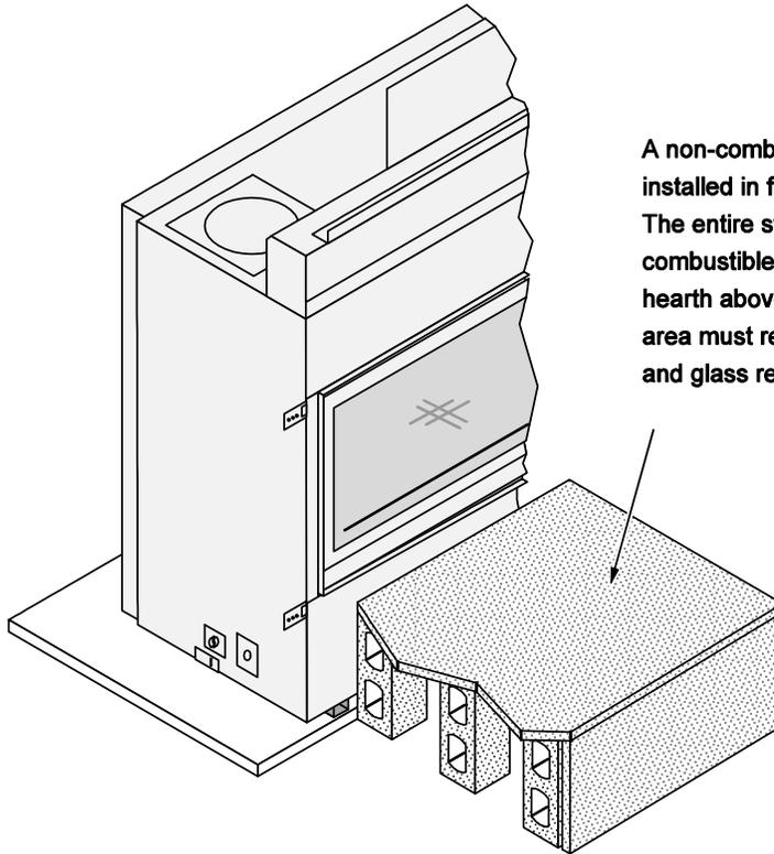
A non-combustible hearth may be installed in front of the fireplace. The entire structure must be non-combustible. Do not build the hearth above the glass opening (this area must remain open for screen and glass removal).
