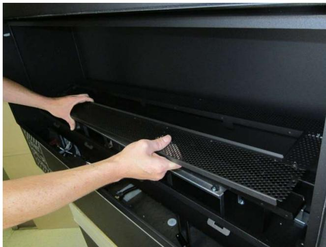
3. Remove the burner. It is held in place with 6 screws (1/4" nutdriver).
