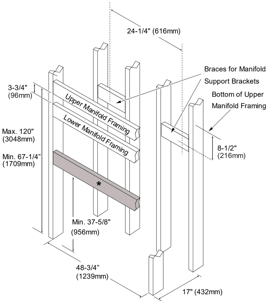
\* The dark-shaded framing may be installed after the fireplace is put into position. It is used to provide support for the facing above the fireplace and nailing brackets.
