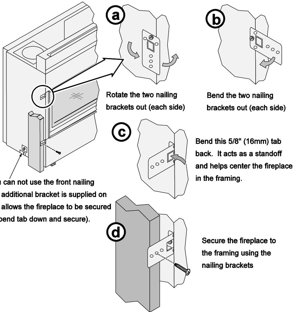
**NOTE:** if you can not use the front nailing brackets, an additional bracket is supplied on the side that allows the fireplace to be secured to the floor (bend tab down and secure).
