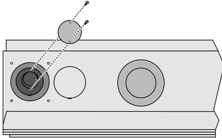
4. Once the third layer is removed, a final cover plate will be visible. Use a 1/4" nutdriver to loosen the screw securing the plate. Reach in and rotate the cover plate to uncover the final hole.
