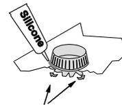
Bend the tabs on the bottom of the starter collar up to lock it in place.
