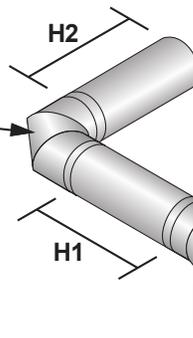
Horizontal length is calculated by adding both lengths of horizontal run (Horizontal Length = H1 + H2).
