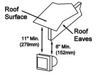
E Minimum 11" (279mm) clearance below unventilated soffits or roof surfaces
