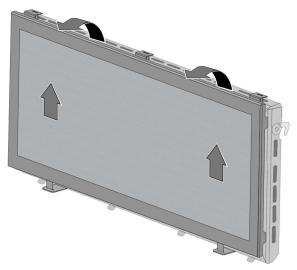
• Lift the bottom tabs out of the brackets on the bottom of the glass frame assembly and remove the barrier screen from the fireplace.
