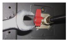
2. Remove the screw that holds the shutoff valve plate in place (1/4" nutdriver). Remove the shutoff valve plate.
