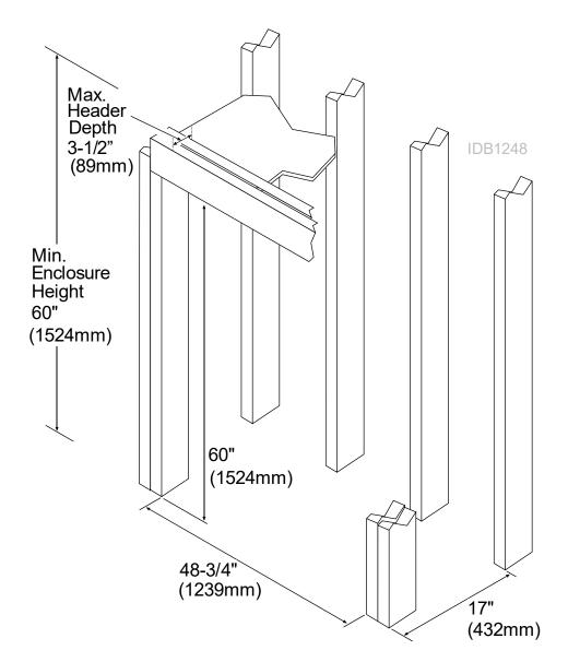
The fireplace enclosure must be a minimum 60" tall (do not build into the fireplace enclosure)
