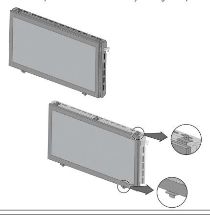
• Lift up on the barrier screen assembly until the top brackets are clear of the tabs on the glass frame assembly. Direct the top edge of the barrier screen forward
