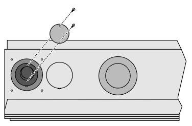
4. Once the third layer is removed, a final cover plate will be visible. Use a ¼" nutdriver to loosen the screw securing the plate. Reach in and rotate the cover plate to uncover the final hole.
