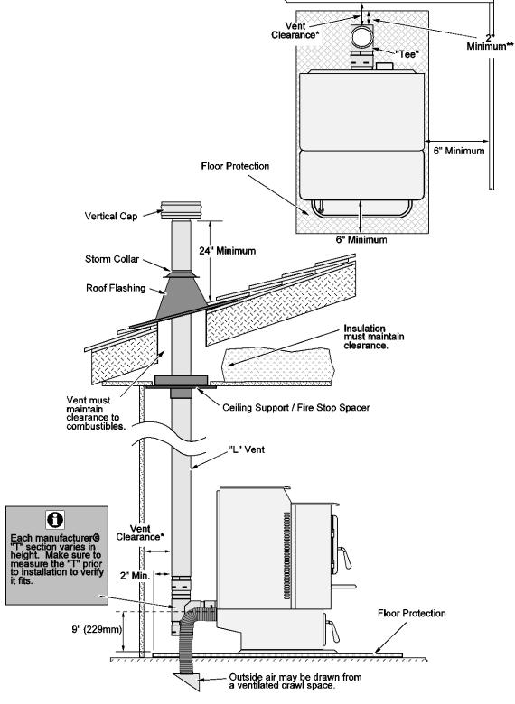
\* Install vent at clearance specified by the vent manufacturer.
