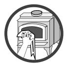
Maintain the door and glass seal and keep them in good condition. Do not operate this heater with broken or missing glass.
