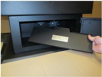
These hooks hold the duct cover in place.
