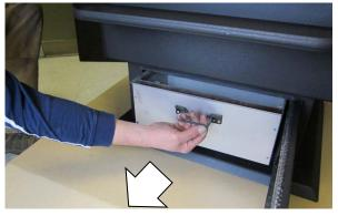
3. Remove the ashpan from the appliance and properly dispose of the ashes (see "Disposal of Ashes" on page 32 for details). You may wish to clean the area below the firebox.
