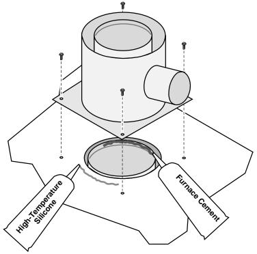
Use high-temperature silicone to seal the anchor plate.
