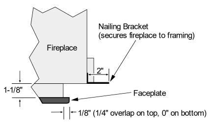
NOTE: Setup face is 1/16" wider on each side and top
