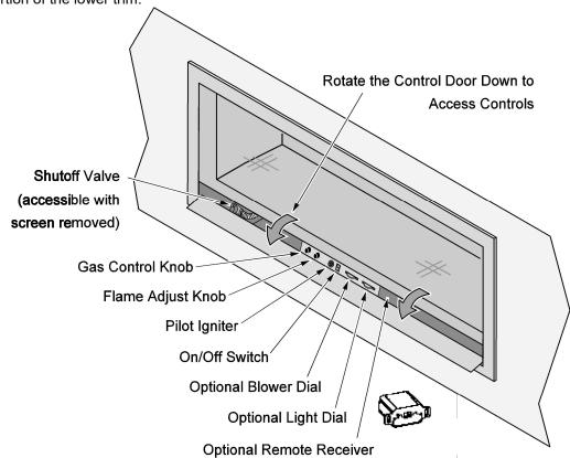
On/Off Switch This control is used to turn the heater on and off.
