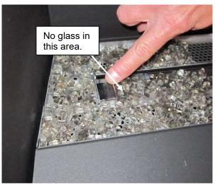
Make sure the rear and end air channels are free of crushed glass. Use a screwdriver to clear this area. **Make sure the glass is only 1 layer deep on the burner.**
