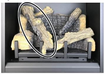
Install log #7 as shown below. The burnt end of the log points toward the center of the burner. Make sure the log does not cover any burner holes or creates any flame impingement.
