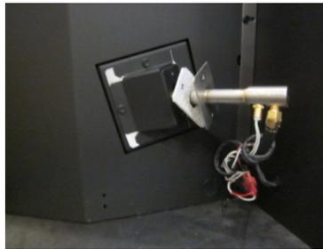
Connect the compressor hose to the igniter as shown and secure with the included hose clamp.
