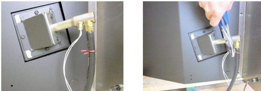
Connect the igniter wires. Orientation of the wires does not matter. Wrap the wires around the compressor hose.
