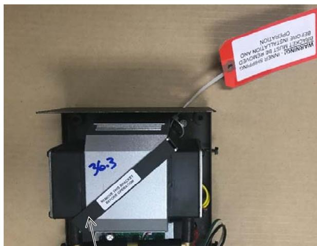
Remove the cover from the compressor assembly. Remove the shipping bracket and discard it along with the 2 screws that held it in place (1/4" nutdriver). Replace the cover.
