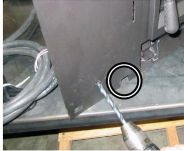
Route the igniter cord through the "mouse hole" in the left side of the panel as shown above. Attach the faceplate to the panel.
