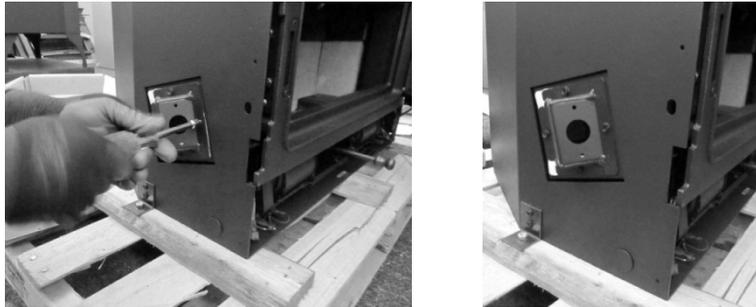
Attach the igniter assembly to the housing using the screws provided, as shown below. Note that the igniter gasket is placed between the housing and igniter assembly.
