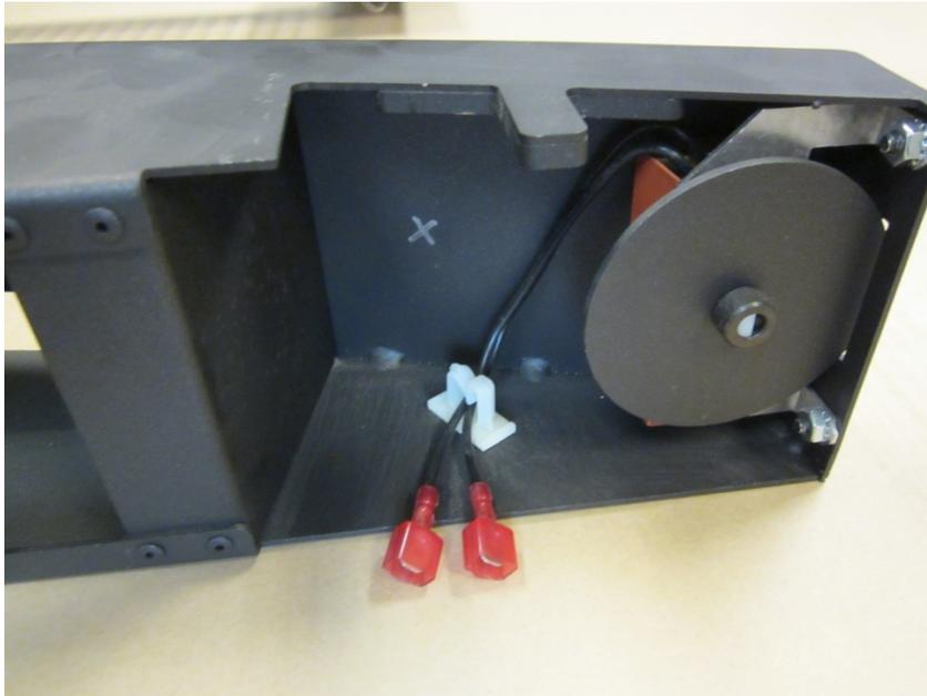
Affix the GreenStart sticker over the hole, and then insert the color-coded start button wires through the hole. The start button should be flush with the trim panel.
