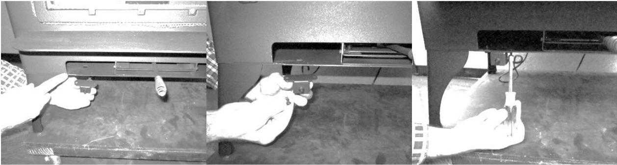
10. Insert the 2 cable holders in the 2 holes on the underside of the stove. Route the start switch wire under the stove, through the cable holders.
