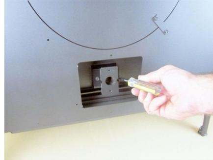
8. Attach the igniter with gasket to the igniter sleeve using the screws and gasket included in this kit. Note that the igniter gasket is placed between the sleeve and igniter assembly.
