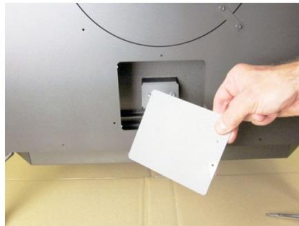
6. Remove the igniter cover plate and gasket. Retain the gasket and screws.
