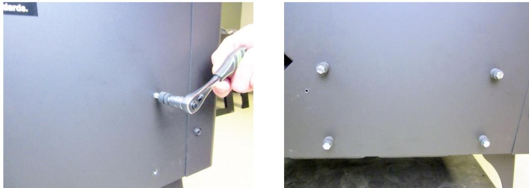
3. Hang the compressor assembly on the rear of the stove, as shown below. The 4 slots fit over the 4 bolts in the grommet notch (see below).
