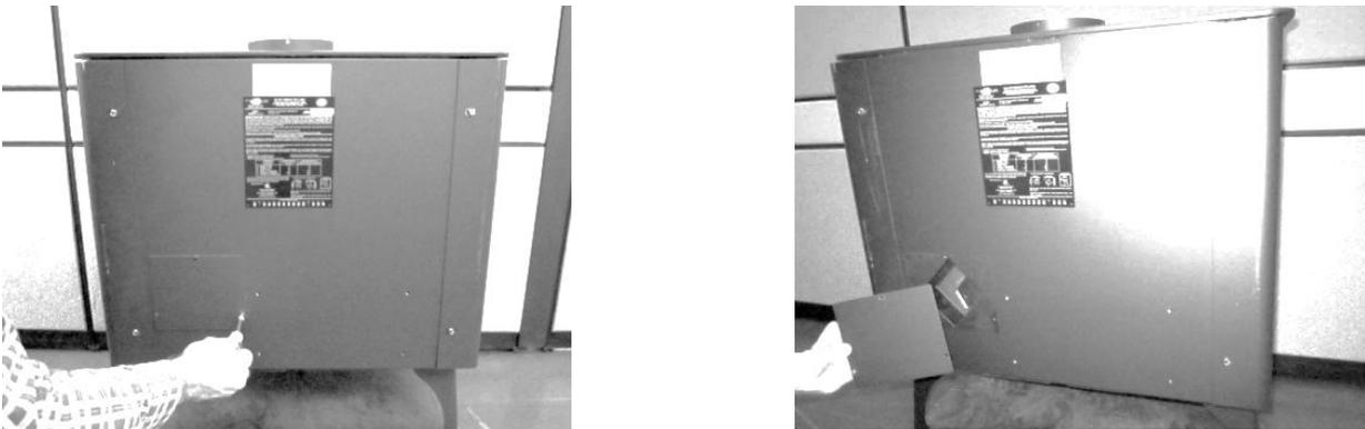
3. Remove the convection chamber cover plate and gasket, as shown below. Retain the screws and gasket.
