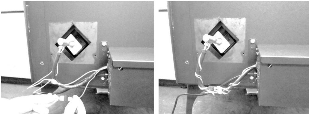
8. Attach the cover box to the heat shield as shown below, using the screws removed in step 2. If your unit does not include these holes, drill the holes with the included bit.
