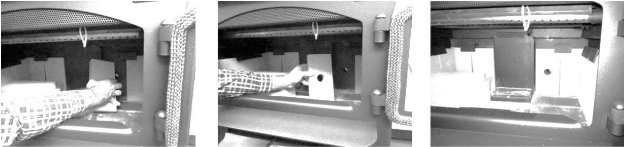
2. Remove the cover plate from the rear of the stove as shown below. Retain the screws.
