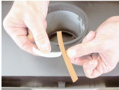
5. While pushing the heat shield back, insert the gasket between the heat shield and heat shield support. Affix the gasket to the heat shield. The photo at right below shows the gasket properly placed.
