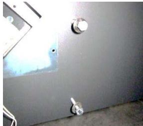
NOTE: The washers are used as spacers, and are inserted between the stove and the compressor assembly.
