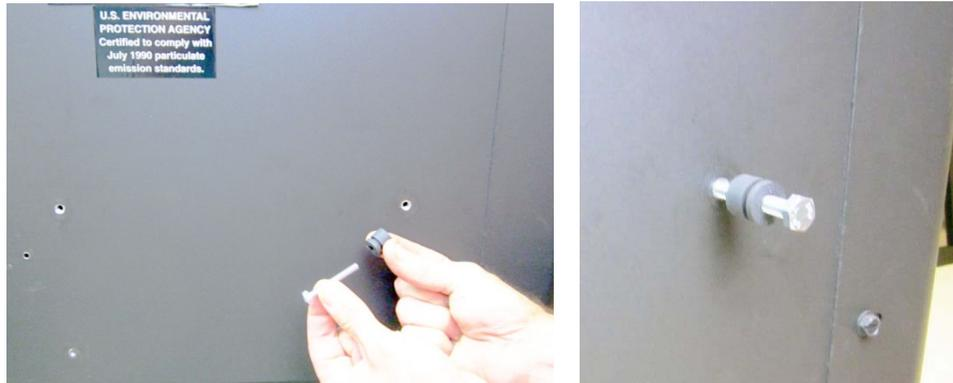
2. Tighten the bolts until the grommets contact the heat shield.
