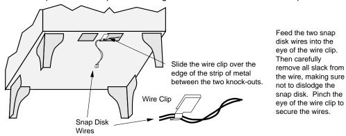
The wires must be properly secured to prevent them from contacting the firebox and shorting out the blower circuit.
