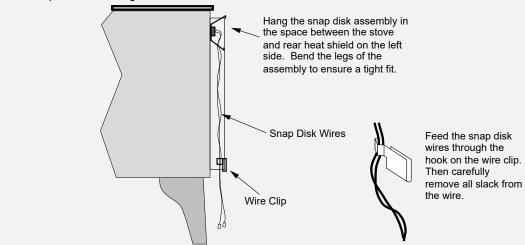
Secure the snap disk wires in place following the directions below.
