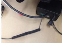
Place the longer piece of loom over the wires and tube leading to the igniter.
