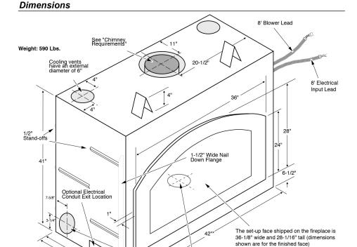
6" Blower hook-ups are on both sides and on the bottom (centered 7-5/8" from the rear edge). Remove the cover
