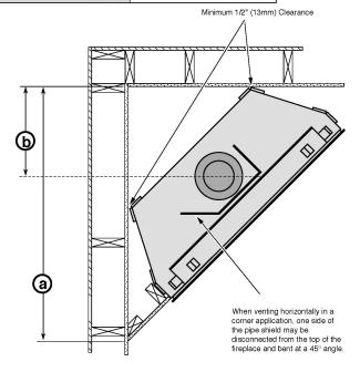
The fireplace enclosure must be a minimum 68" (1728mm) tall. Do not build into the fireplace enclosure.
