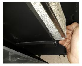
3. Install new combustor making sure that the <u>side insulation</u> and the <u>combustor top and bottom</u> <u>gasket</u> are in place.
