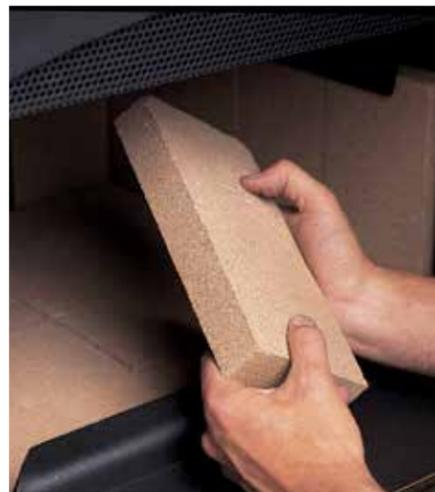
We use real kiln-fired, refractory firebrick in the firebox. This is the same material used to line commercial boilers and furnaces, and is twice the weight of typical brick. The brick protects the steel while increasing the internal temperature within the firebox.
