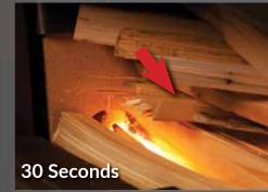
Hot surface igniter blows 1,400 degree heated air into the firebox, igniting the wood.
