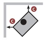
A - Stove to Sidewall 10" (254mm) B - Stove to Backwall 5" (127mm) C - Stove to Corner 5" (127mm)
