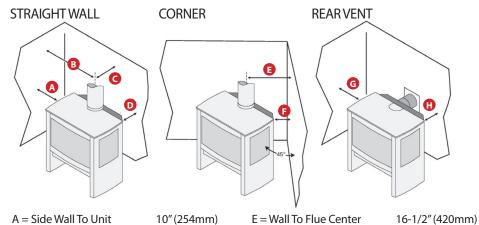
A = Side Wall To Unit B = Side Wall To Flue Center 25-1/8" (638mm)C = Back Wall To Flue Center 6-7/8" (175mm)D = Back Wall To Unit
